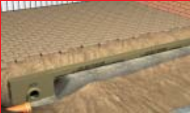
3. Lay channels starting at outlet. Set a string line at required height to ensure level.
